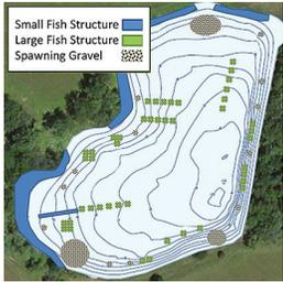
An accurate waterbody map provides the information needed to get the most out of your fishery. Lake bathymetric mapping can help determine the areas likely to be used by diverse species of fish at various stages in their life-cycle, so that we can accurately manage, strategically place structural cover, and most importantly, help to find out where those trophy bass are hiding!
