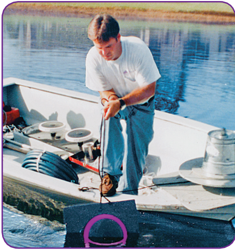
Placing Vertex AirStation™ into Heron Cay's lake.
