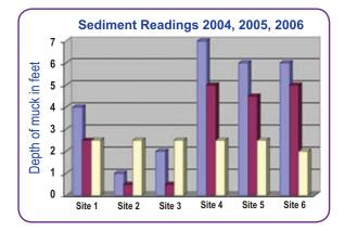
By April 2005, the oxygen level had increased to 10.4 mg/l, clearly satisfying the BOD, which was determined to be 0.23 mg/l. The average level of muck at the 6 sites was 3.0 feet. Minimum amounts of 0.5 feet were recorded at 2 sites while the maximum level of 5 feet was recorded at another site. Since installation, the average level of bottom muck has decreased by 30.2%.
