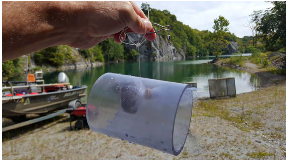
Figure 4. Example of a cage stocked with 20 adult mussels and ready for deployment.
