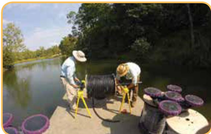
*A submersed aeration system can help oxygenate the water column in deeper lakes and ponds. These systems improve vertical mixing at depths where water is not naturally stratified by using an on-shore compressor to pump oxygen to the bottom of the waterbody.*
